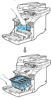
6 Release the gray lock lever (1) that is on the left side of the machine. Lift the front of the drum unit and pull the drum unit completely out of the machine using the green handles on the drum unit.
